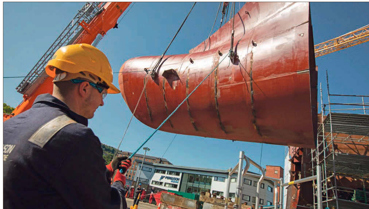
The bulbous bow is attached to Hull 802 at the nationalised Ferguson Marine shipyard at Port Glasgow.
