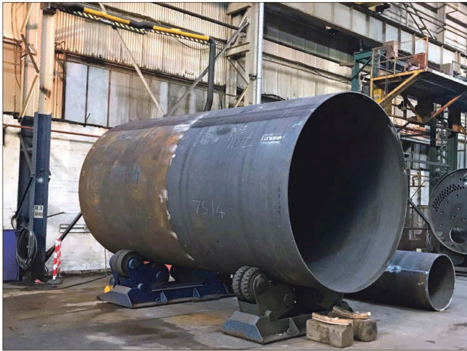
Waverley's new boilers take shape at the yard in Annan.
