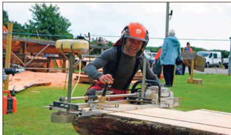
Jamie Campbell demonstrates his Alaskan mill, a mobile chainsaw mill that can be operated by a single person. 01_B34wood11
