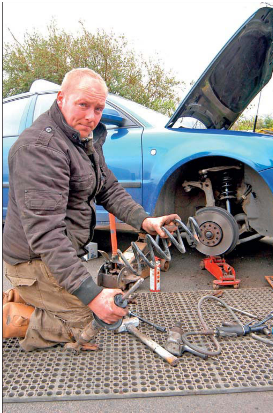
Mechanic Craig Galloway with the broken spring and shock absorber on Willie McDonald's taxi. b17pot01
