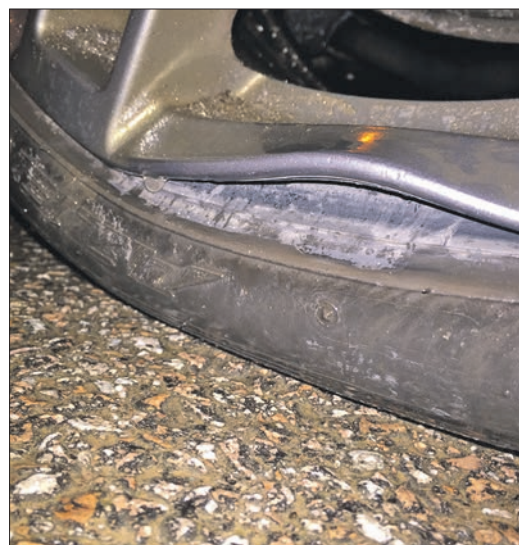
Charlene Glencross hit a pothole in Airdrishaig, buckling an alloy wheel on her car.
