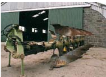
A modern farm building with a six furrow reversible plough sitting outside.
