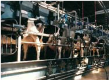
A milking parlour with the teat cups ready to milk the cows.
