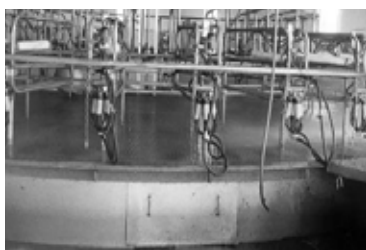
A rotary milking parlour. The cows get milked at the parlour slowly moves around.
